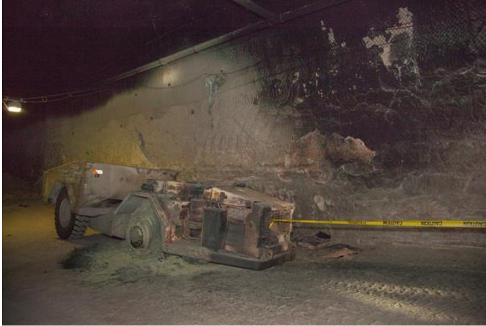
Figure 22: Haul Truck and Rib Spalling
