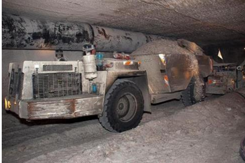
Figure 4: EIMCO 985T 15 Haul Truck (74-U-006A)
