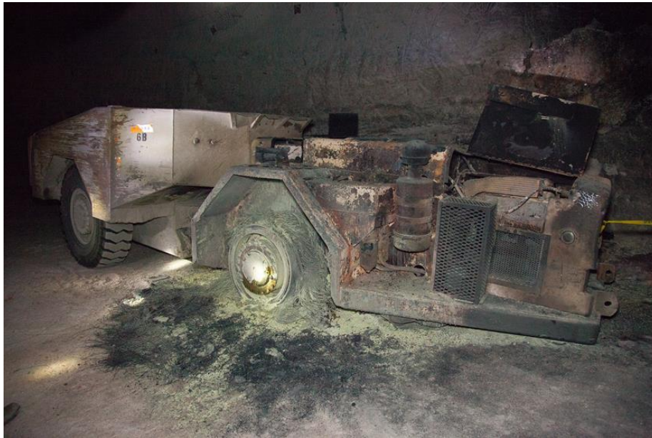
Figure 21: Salt Haul Truck Damage (Engine Cowling Was Opened Post-Fire)
