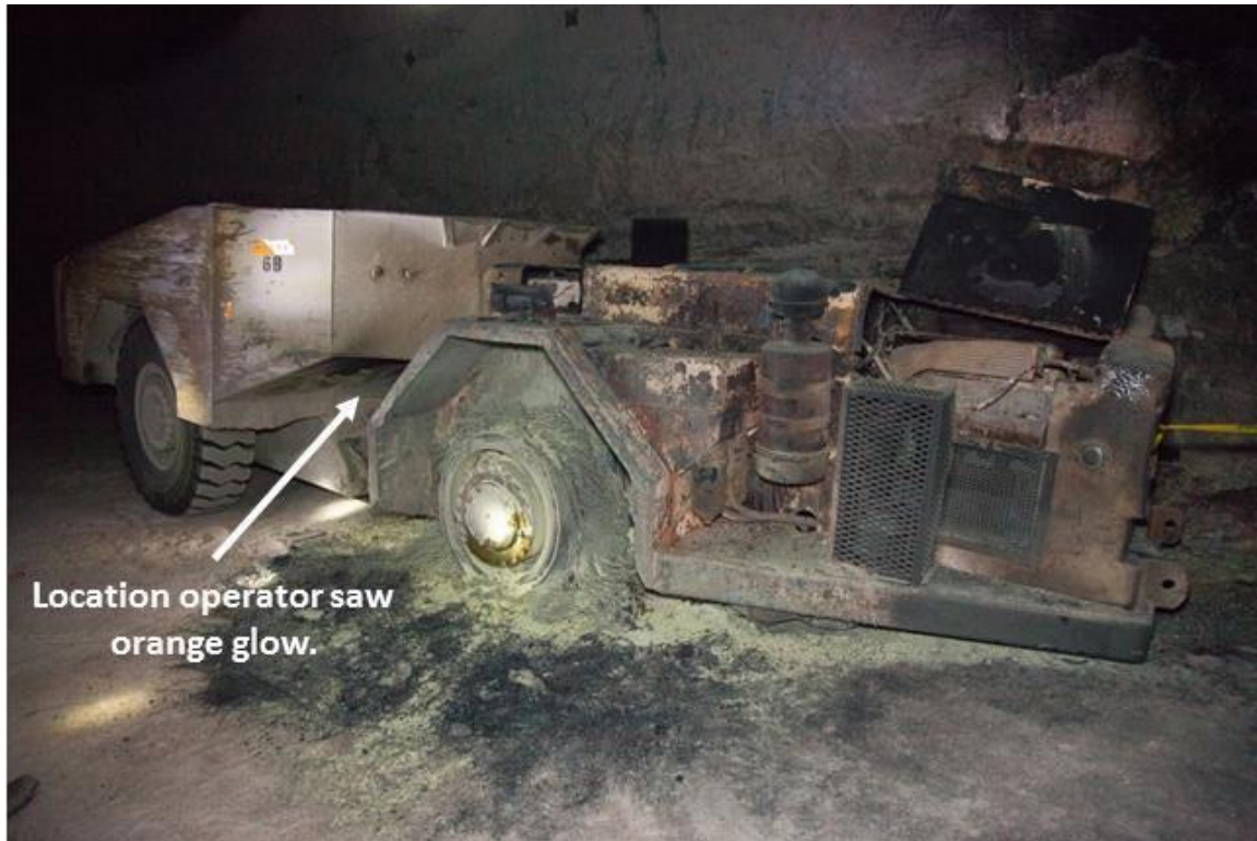
Figure ES-1: EIMCO Haul Truck 74-U-006B after Fire
