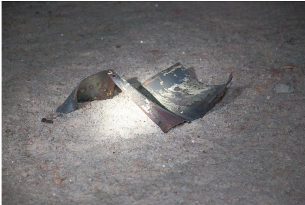
Figure 26: Damaged Access Plate
