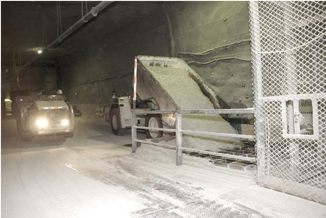
Figure 7: The Loading Pocket “The Grizzly”
