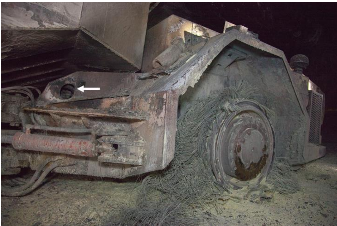
Figure 9: Photo Showing the Area on the Salt Haul Truck where the Fire Extinguisher was Discharged
