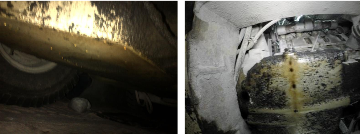
Figure 13: Buildup of Engine Fluids on the Underside of Vehicles in the Mine
