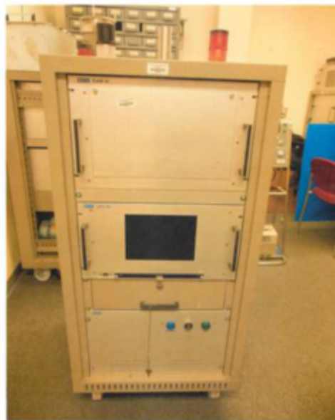
Figure ES-1: RADOS Continuous Air Monitor
