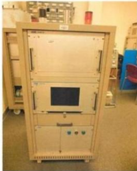
Figure 6-47: RADOS Continuous Air Monitor
