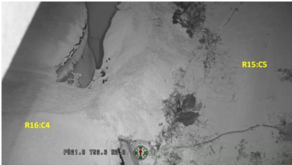
Figure 6-42: Bridge between the R15:C5 SWB Lid and R16:C4
