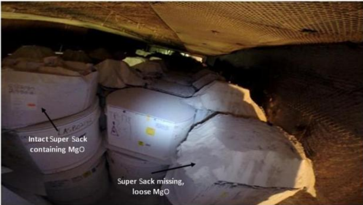
Figure 2-2: Missing Super Sacks Leaving Loose Piles of MgO on Waste Stacks
