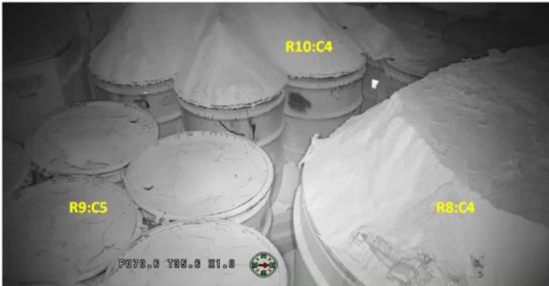
Figure 6-22: Damage at R9:C5 and R10:C4
