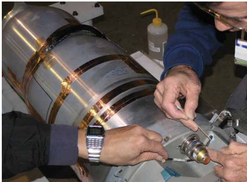
Figure 2-3. Technicians attach instrumentation to the exterior of a W80 Environmental Test Unit.
