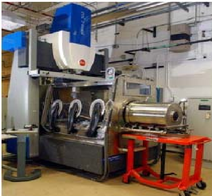
Figure 7-3. Coordinate Measuring Machine in glove box is used for machining and inspecting parts.
