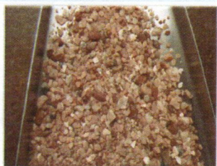
Granitic cuttings from 2860 to 2870 ft. from well 30-037-20027. #1 RC Bell, Sun Exploration & Prod Co, 1982.
