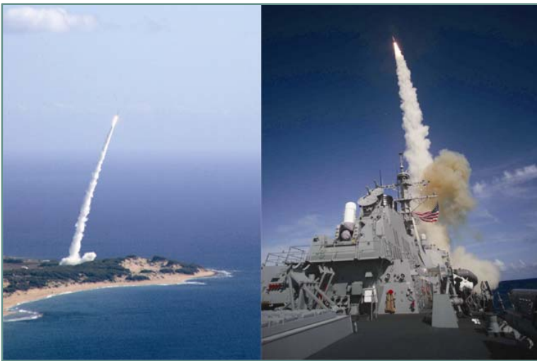
A medium-range ballistic missile with a separating target is launched from the Pacific Missile Range Facility on Jun. 22, 2007 (left photo). Minutes later, a Standard Missile (SM-3) was launched from the Aegis combat system equipped Arleigh Burke class destroyer USS Decatur (DDG 73), successfully intercepting the ballistic missile threat target (right photo). It was the first time such a test was conducted from a ballistic missile defense equipped-U.S. Navy destroyer. U.S. Navy photos.
