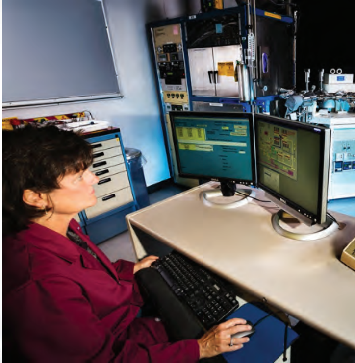
Sector Mass Spectrometer optimized for gaseous isotopes.
