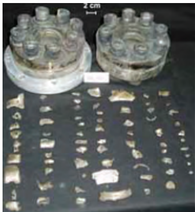
Predictive modeling with validation experiments of HE thermal cook-off events.
