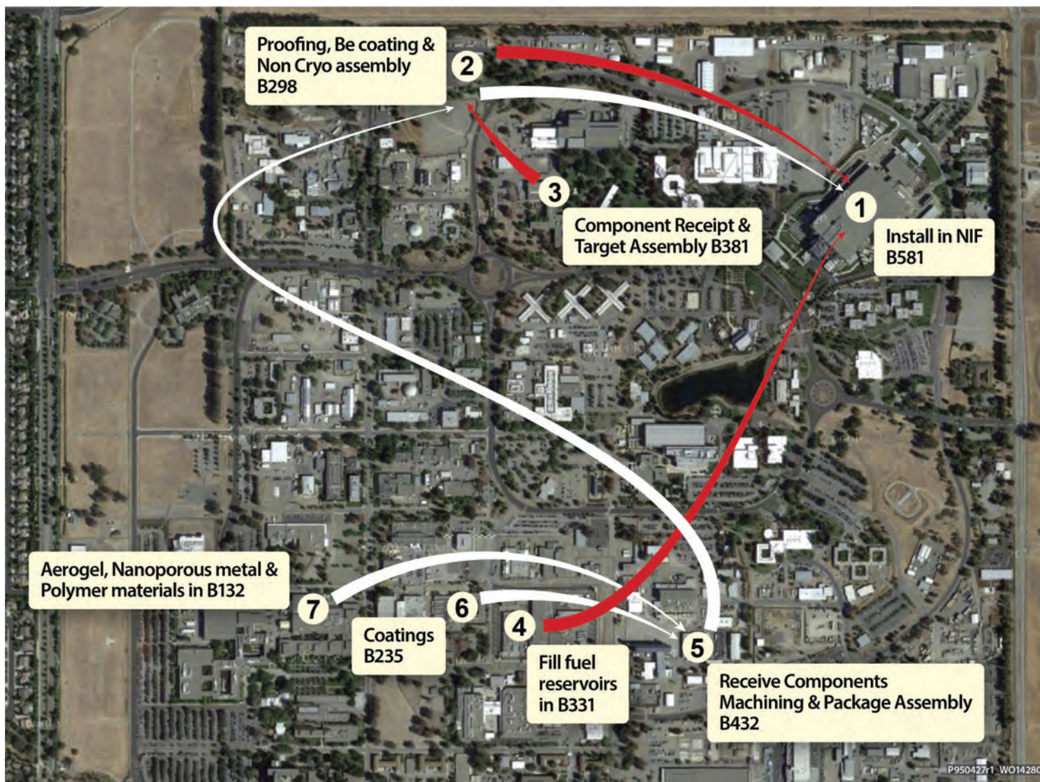
Current operations for NIF target fabrication are disjointed, requiring movement of targets amongst several facilities during the process. The consolidation into B298 would eliminate the need to transfer targets/components to and from B432.
