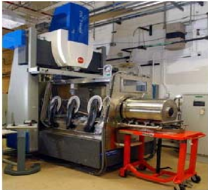
Figure A-7-2. Coordinate Measuring Machine in glove box is used for machining and inspecting parts.
