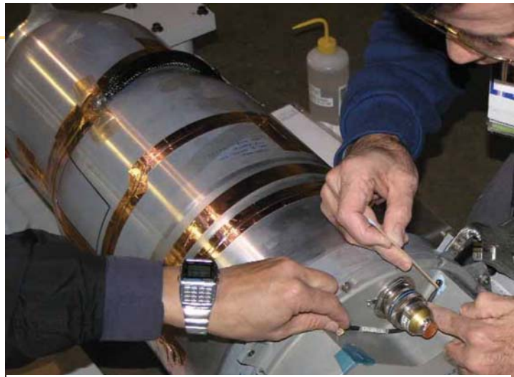
Figure A-2-3. Technicians attach instrumentation to the exterior of a W80 Environmental Test Unit.
