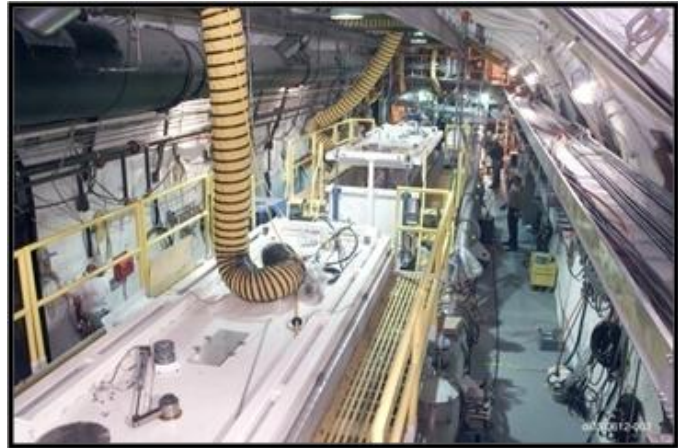
Figure A-3-2. Cygnus dual-beam radiographic source enables X-ray imaging of Subcritical experiments.
