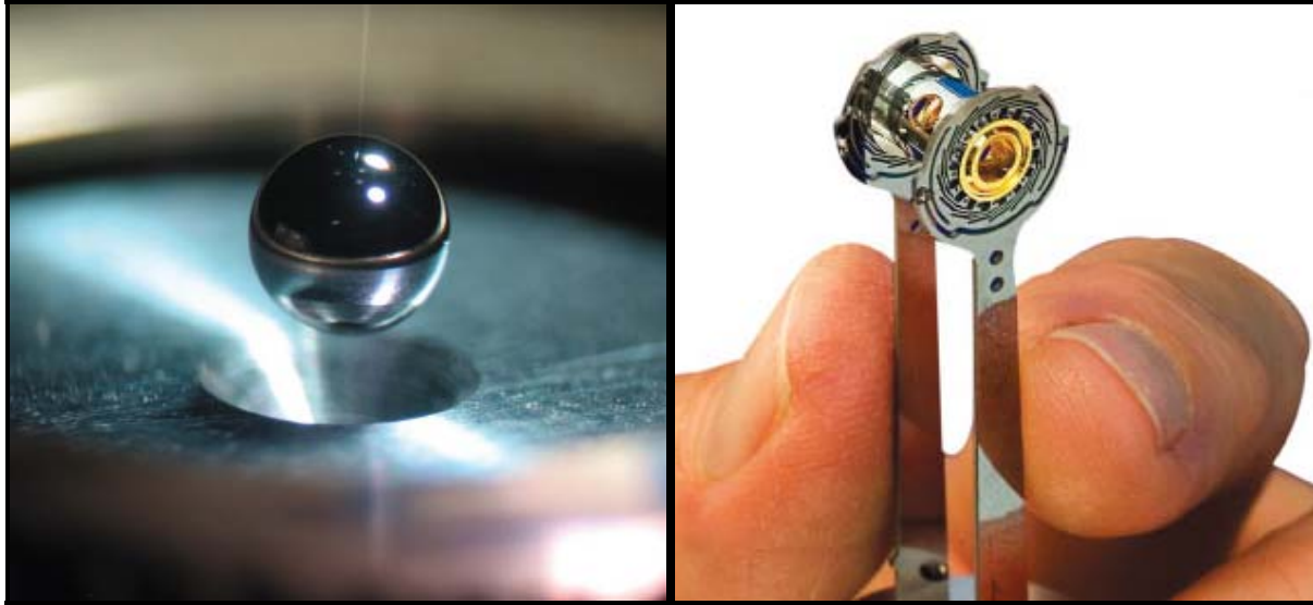
Figure A-5-7. ICF Target components. Left panel: The polished beryllium capsule is 2 millimeters in diameter and holds the cryogenic DT fuel. The 10-micrometer fill tube attached to the top of the capsule is barely visible. Right panel: The thermomechanical package for the hohlraum-capsule assembly.
