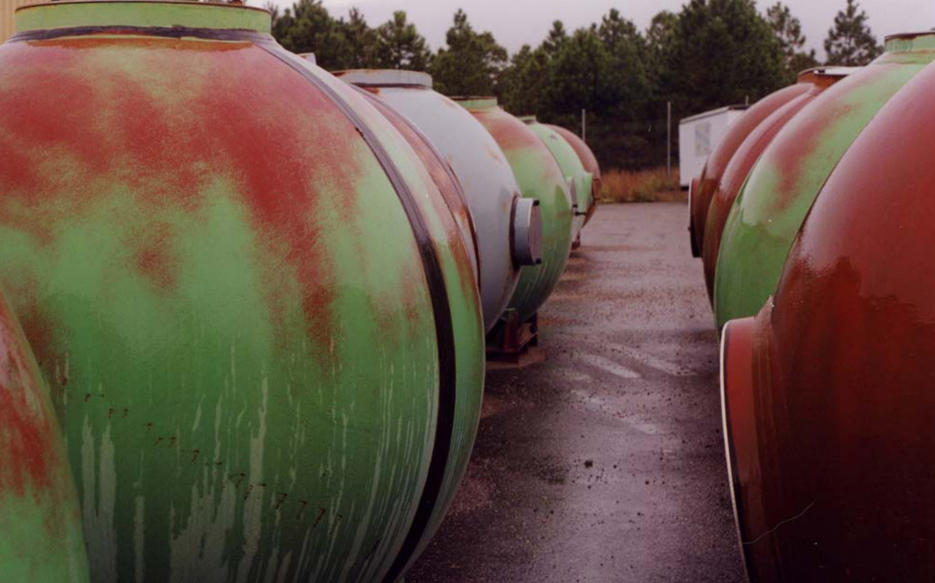
“Appaloosa”/“Dynex” vessels at LANL TA-60 – for pit explosive “subcritical” pit testing above-ground using real Pu-239 or Pu-242. These are single-axis vessels.
