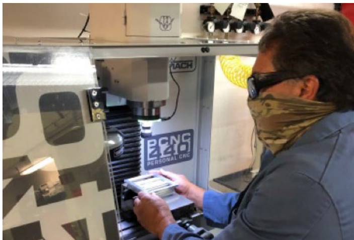
Gio Romero fabricates one of many unique plutonium experimental sample holders.
