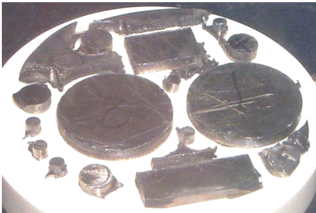
Figure 7 Specimens are rough cut from the disk
