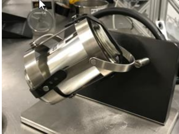
Figure 2-9. Blending of Plutonium Oxide and Adulterant in a Blend Can
