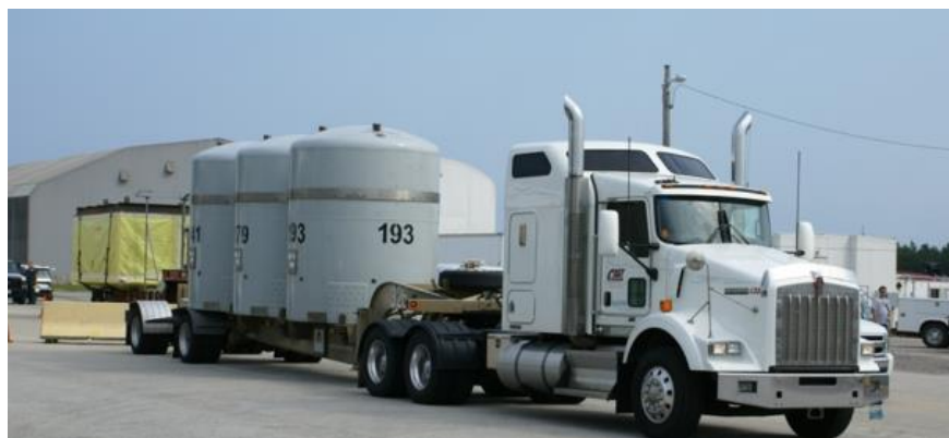
Figure 2-13. TRUPACT-II Transporter Used for Shipping CH-TRU Waste to the WIPP Facility
