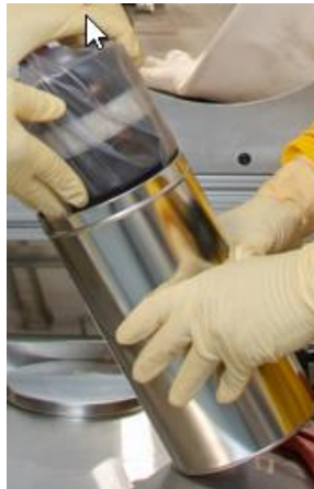
Figure 2-10. Diluted Plutonium Oxide CH-TRU Waste Packaged in a Can/Bag/Can
