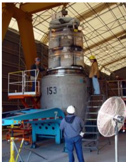
Figure 2-12. Drums Loaded into a TRUPACT-II for Transport
