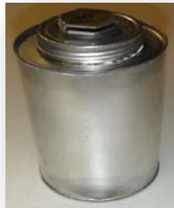
Pu oxide is placed in new can along with dry inhibitor to dilute Pu to less than 10 weight percent
