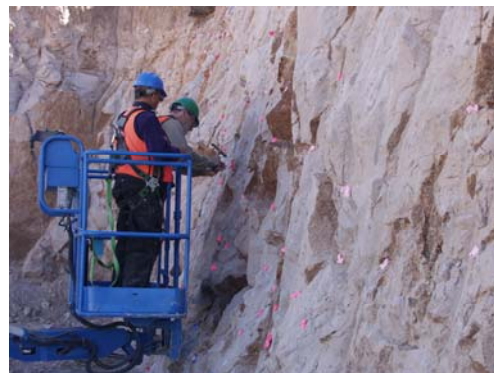
▲ Installing color-coded flagging to demarcate geologic features
